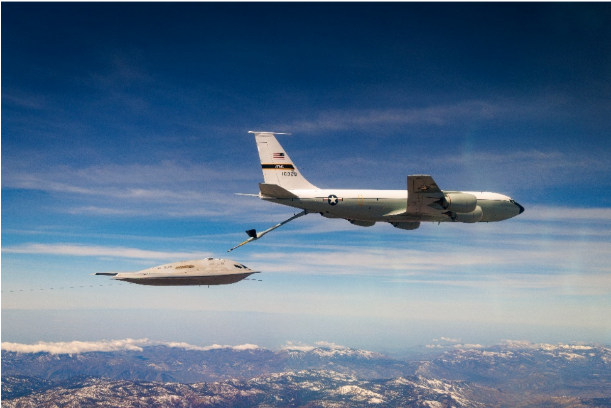
The B-21 Raider conducts aerial refueling with a KC-135 Stratotanker, which is a key part to the Raider's role in projecting power globally. (Photo
