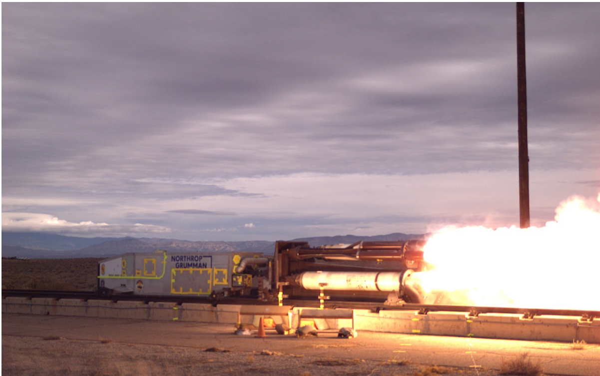
Sentinel's Guidance and Control (G&C) hardware has passed an initial mass model sled test conducted by Northrop Grumman Corporation and the U.S. Air Force. (Photo Credit: U.S. Air Force)
