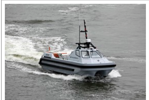
The Northrop Grumman AQS-24B towed mine hunting sensor on the Atlas Elektronik ARCIMS Unmanned Surface Vessel (USV). The AQS-24B features the only high speed synthetic aperture sonar for mine detection, localisation and classification, and an optical laser line scan sensor for mine identification.
