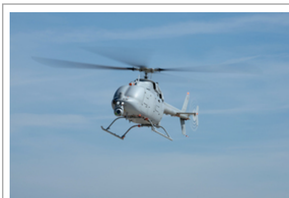
The MQ-8C Fire Scout completes a test flight at the Point Mugu Sea Range, Naval Base Ventura County. This flight was one of 11 operational assessment events to validate the system's performance, endurance and reliability. (Photo by Northrop Grumman)
