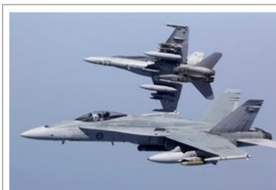
The Royal Australian Air Force flies the Northrop Grumman LITENING advanced targeting pod on its F/A-18 aircraft as the Hornet Target Designation System. Photo courtesy of the Royal Australian Air Force.
