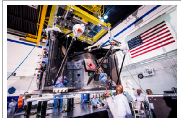
Northrop Grumman completes manufacturing and assembly of the spacecraft structure, or bus, for NASA's James Webb Space Telescope. The bus houses the spacecraft's propulsion, electrical power and communications, and it will help take the Webb Telescope 1 million miles from earth.
