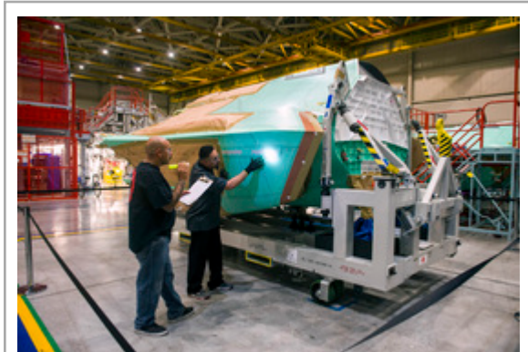
Northrop Grumman quality team at the company's Palmdale Aircraft Integration Center of Excellence performs final inspection of AX-5 center fuselage before its delivery to Japan's F-35 Final Assembly and Check Out facility in Nagoya, Japan
