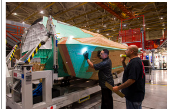
Mechanics from Northrop Grumman's F-35 program team in Palmdale, Calif. check the quality of workmanship that went into producing AX-5, the center fuselage that will become a central part of the first F-35 Joint Strike Fighter assembled by Japan
