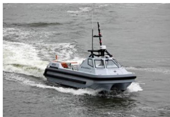
The Northrop Grumman AQS-24B towed mine hunting sensor on the Atlas Elektronik ARCIMS Unmanned Surface Vessel (USV). The AQS-24B features the only high speed synthetic aperture sonar for mine detection, localisation and classification, and an optical laser line scan sensor for mine identification.
